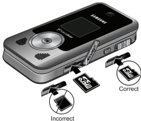
3. Press the memory card into the slot until the card locks into place.
