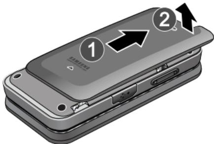
3. Lift the bottom of the battery up (1) and away (2) from the phone.
