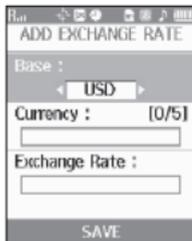
4. Use the Left and Right navigation keys to select the Base currency to be converted from.
