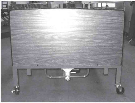
fig 1: casters mounted at standard height
