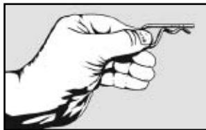
Close-up of Hair Pin Clip (#6) inserted into hole in Clevis Pin (#7)
