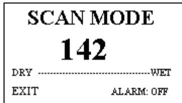
3. You may begin taking readings by firmly pressing the back of the meter onto the material to be tested. This will display a relative reading that ranges between 0 and 300.
