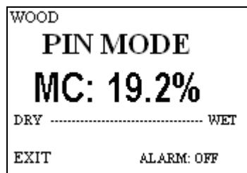
3. Push the contact pins into material to be tested. Any Delmhorst electrode may also be used in **WOOD** mode by simply attaching it to the connector next to the contact pins.
