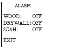
3. After the alarm is turned on, use the  $\Rightarrow$  key to increase the alarm value, and the  $\Leftarrow$  key to decrease alarm value.
