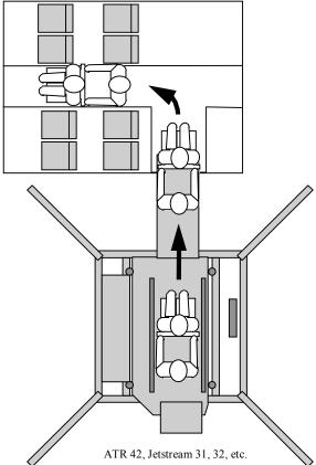
When the passenger and attendant are positioned properly on the deck with the wheelchair brakes locked, the deck gate [44] is then closed and relatched. The passenger should keep their arms on their laps in front of them to avoid interference with the bracing members of the ramps.
