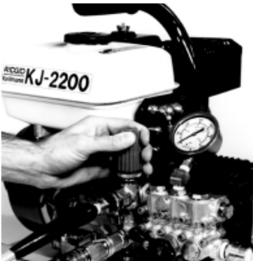
Figure 4 – Adjusting the Unloading Valve
