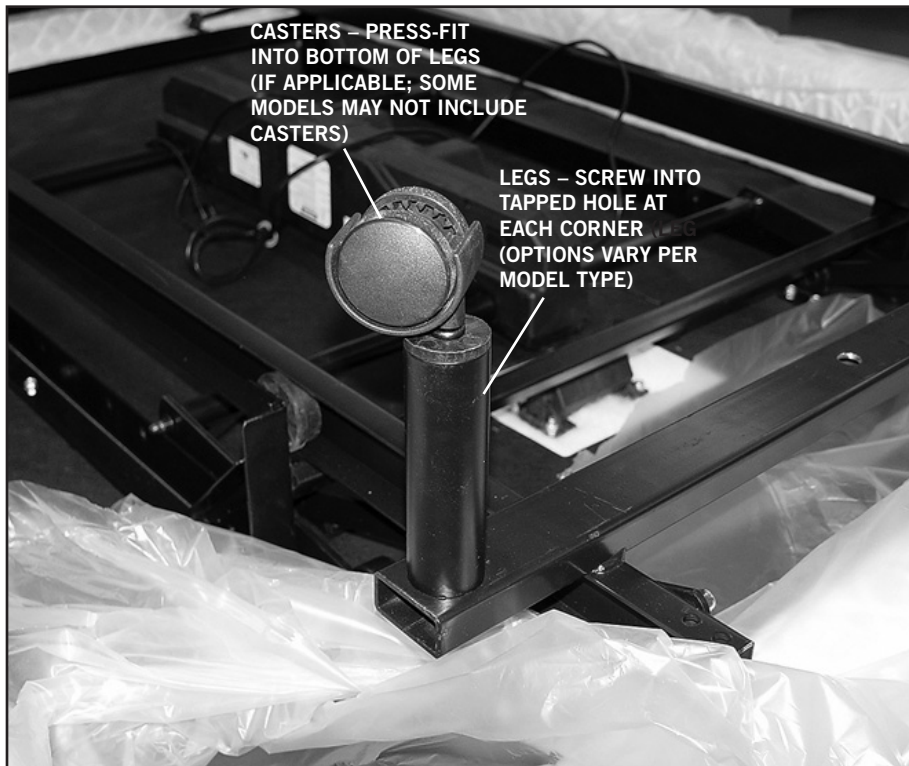
FIGURE 1: Leg installation. Caster installation, if applicable. (Optional 4" leg with caster shown.)
