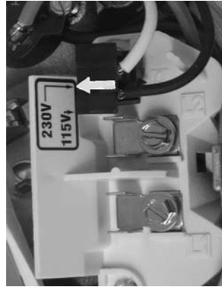
Figure 4A -Voltage Change Plug Set for 230 Volts.
