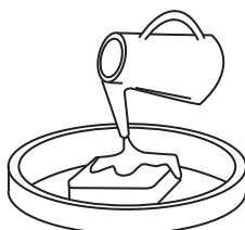
FIGURE 34: Wash Air Filter
