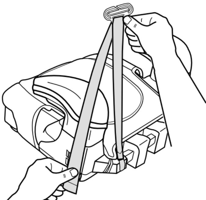
3. Slide the vehicle shoulder belt onto the clip as shown in 4 and pull strap down to tighten clip against child's shoulder.
