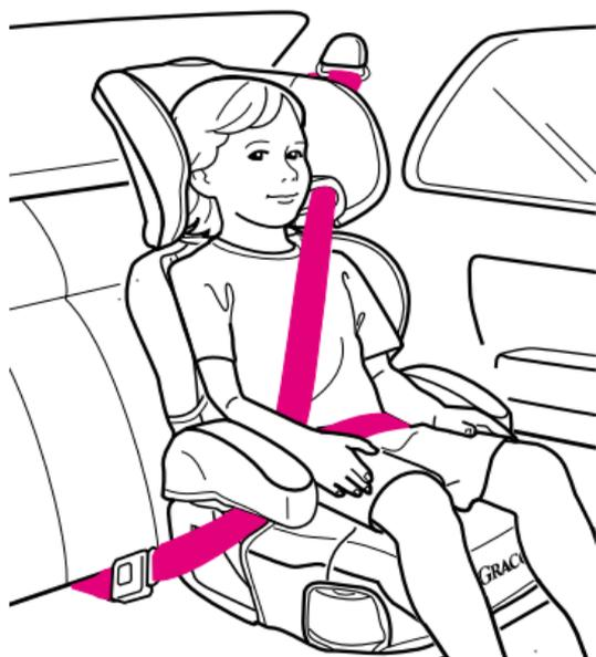
3. **Position shoulder belt through the shoulder belt guide shown in ②, NOT as shown in ③. Fasten buckle and pull up on the shoulder belt to tighten.**
