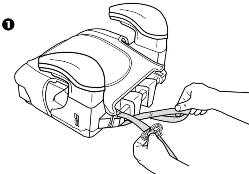
2. Pass the clip and strap through the loop end as shown in **2** and pull strap up **3** .
