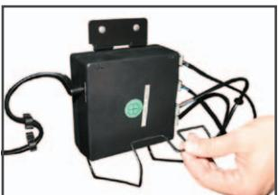
To remove control box, release metal clip and unplug cords.
