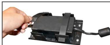
To remove power supply, release plastic straps and unplug cords.
