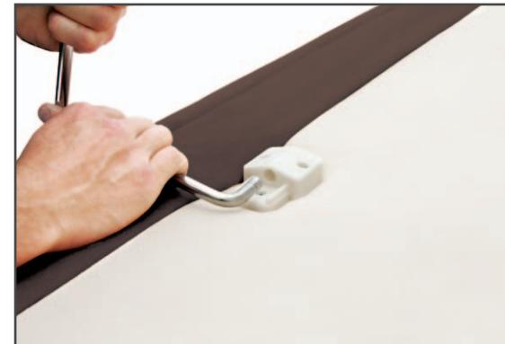
Locate the mattress retainer bar brackets. Slide the left side of the mattress retainer bar into the bracket. Pull the retainer bar to the opposite bracket and secure the right side.
