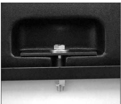
7. From the bottom side slide the Mounting spacer (13), washer (4) and .500" locknut (6) to the bolt assembly.
