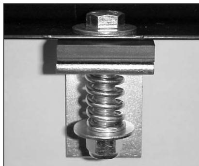
5. With all four angle brackets secured to the mounting base it is time to tighten the lock nut until the compressed length of the spring is 1.500". **DO NOT** completely compress the spring.
