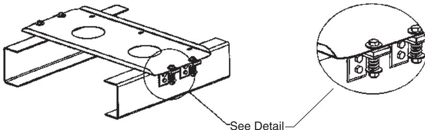
2. Mark the position of the angle bracket on the frame rail. You will need to drill two holes per bracket to attach the angle bracket to the frame rails. Use eight .500" diameter capscrews that are grade 5 or better along with lock nuts to attach the angle brackets to the frame. **CAUTION:** Before drilling any holes, make sure there is adequate clearance on both sides.
