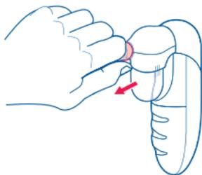
Separate the suction portion of the aspirator from the base by placing thumb under tip and peeling it off the aspirator.
