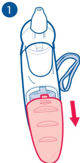
Remove the battery compartment cover as shown.
