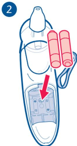
Insert two (2) AA (LR06) alkaline batteries matching positive (+) to positive (+) and negative (-) to negative (-).
