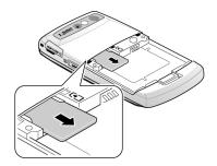
**6.** Place the battery so that the 3 brass tabs on the end align with the 3 brass prongs at the bottom of the battery compartment (1). The arrow on the battery should be pointing down. Press the battery down until it clicks into place (2).
