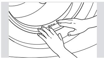
While holding down the door gasket, inspect the interior gasket by pulling it down with your fingers. Remove any foreign objects if found trapped inside this gasket. Make sure there is nothing blocking the holes behind the gasket.
