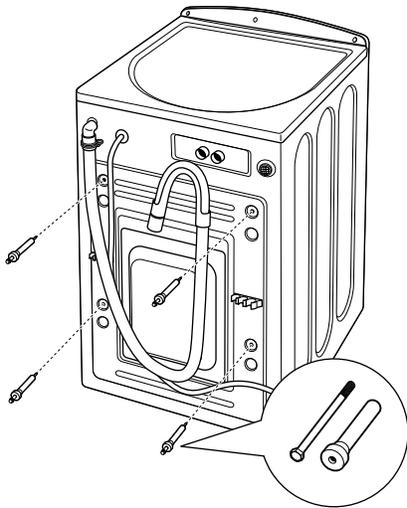
**NOTE:** Failure to remove the shipping braces can cause the washer to become severely unbalanced.
