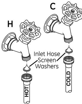
5. Connect the inlet hose ends to the HOT and COLD water faucets tightly by hand, then tighten another 2/3 turn with pliers. Turn the water on and check for leaks.
