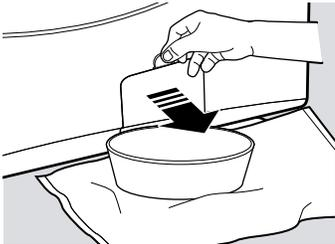
1. Using a coin or flat screwdriver in the notch on the door, open the access door.
