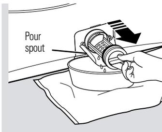
4. Turn the pump filter counterclockwise and remove the filter. Open slowly to allow the water to drain.
