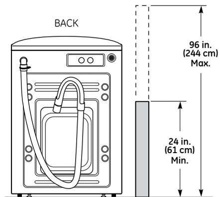
**NOTE:** The drain hose attached to the washer can reach a 58" (147 cm) high standpipe. For a higher standpipe, contact an authorized parts distributor.
