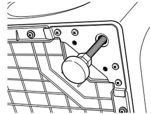
**NOTE:** Keep the leg extension at a minimum to prevent excessive vibration. The farther out the legs are extended, the more the washer will vibrate.
