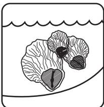
Prolonged exposure to salt water can damage and/or shorten the expected lifetime of this product. The marine environment includes many damaging elements including corrosion, abrasion and damage from marine life such as barnacles. Regular cleaning and rinsing with fresh water can reduce these risks. A PVC-safe antifouling paint should be used to help protect this product against marine growth. **DAMAGE CAUSED BY EXPOSURE TO SALT WATER IS NOT COVERED BY WARRANTY.**
