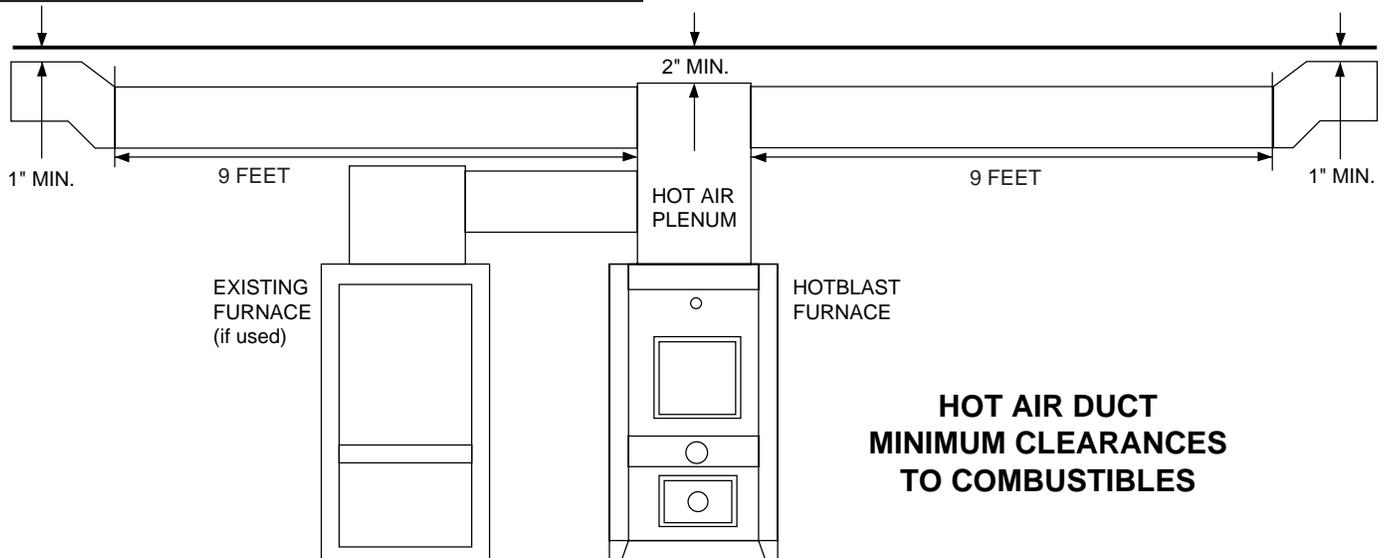
existing plenum at an angle (approximately 45 degrees) will facilitate air flow from the furnace while diverting air from the existing furnace.
