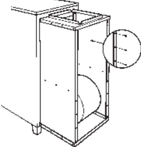
Be sure filter box is perfectly square. Mark position of screw holes on back of furnace. Drill starter holes and secure assembly to back of furnace with self-tapping screws.
