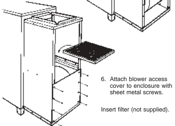
6. Attach blower access cover to enclosure with sheet metal screws.
