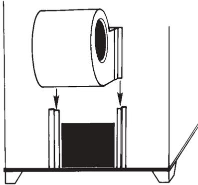
NOTE: Prior to operation, be sure to remove brick retaining strips.
