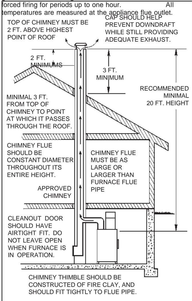
highest point of the house, or 2' above the point at which the chimney is 10' from the roof.
