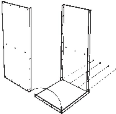
1. Attach sides of filter box to bottom with (4) sheet metal screws per side.
