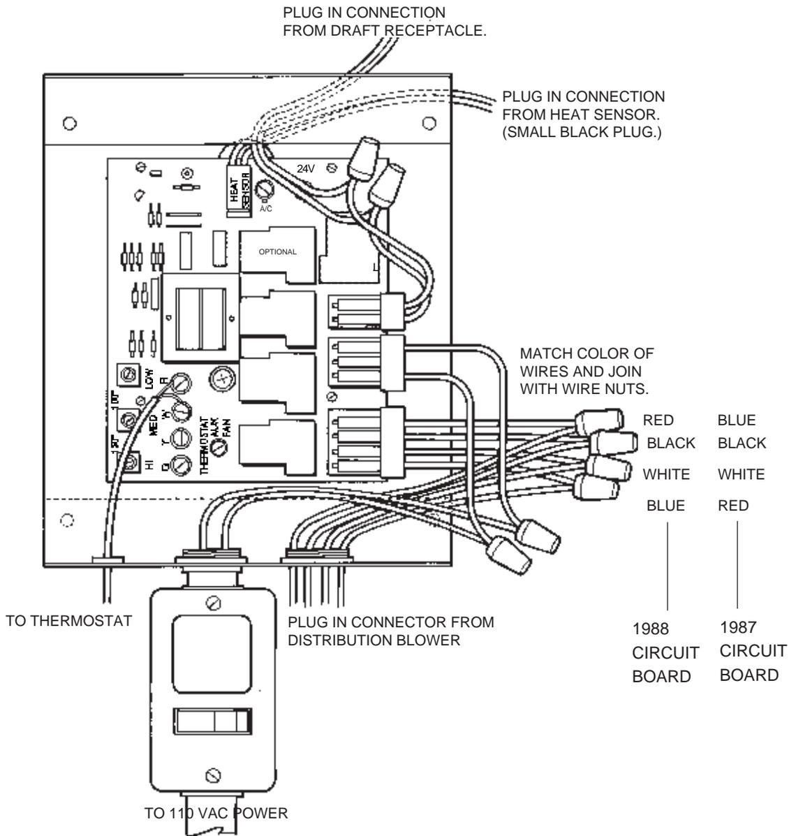
NOTE: DAMAGE TO HEAT SENSOR WILL PREVENT UNIT FROM OPERATING PROPERLY.
