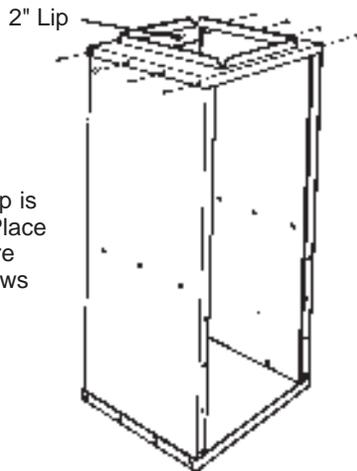
2. Position top so 2" wide lip is turned toward furnace. Place top over sides and secure with (4) sheet metal screws per side.
