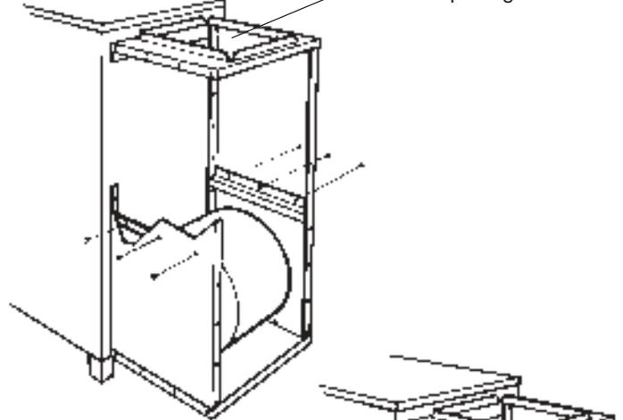
5. Position filter filler between side filter holders and secure to back of furnace with two self-tapping screws.
