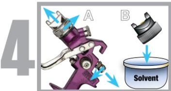
**Disassemble and clean inside of air gun. Soak air cap in cleaner and scrub clean.**
