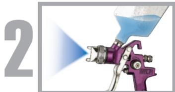
**Fill paint cup with cleaning solvent and spray through spray gun. Repeat until spray shows no paint color.**
