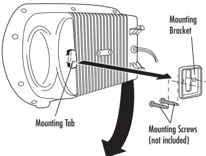
3. Turn heater sideways and position the mounting tab on the back of the heater so it lines up with the mounting bracket.
