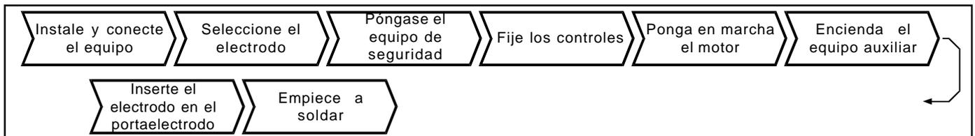
FIGURA 4-7 SECUENCIA PARA SOLDAR CON ELECTRODO REVESTIDO ( SMAW )
