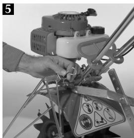
Finally, insert the retaining pin that secures the right and left Plant Guards to the universal holder.
