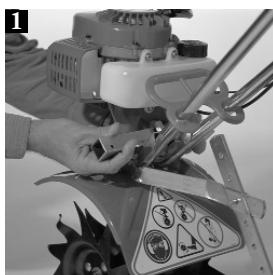
Secure the Universal Holder (key #2) below the fuel tank onto the tiller handles.
