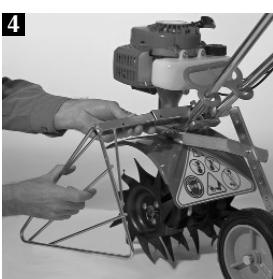
Insert the Right and Left Plant Guard (key #1 & 4) into the universal holder. Make sure that the Plant Guard is facing forward as shown.
