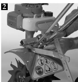
Position the Metal Plate (key #5) below the tiller handles and insert the Bolt (key #6) into the threaded hole in the Universal Holder (key #2).
