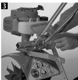
Tighten the Bolt (key #6) until the Universal Holder (key #2) is secured to the tiller handles.
