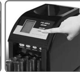
Push the tube tray back to the proper position. Turn on the machine.
