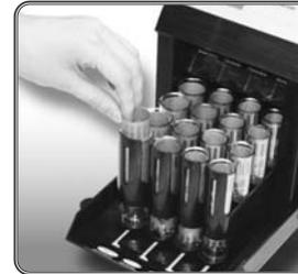
Open front cover on coin sorter and insert preformed coin wrappers into the corresponding coin tubes.
