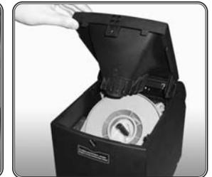
To retrieve jammed items, unscrew Hopper Lid and remove Inner Vessel.
