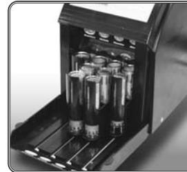
When a coin tube is full, the machine will stop temporarily to slide another coin tube into position.
