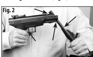
**WARNING:** BE CAREFUL TO KEEP FINGERS CLEAR OF THE COCKING LEVER. GRASP THE COCKING LEVER FIRMLY AS YOU COCK IT AND CLOSE IT TO PREVENT IT FROM SNAPPING BACK AND POSSIBLY CAUSING SERIOUS INJURY.
