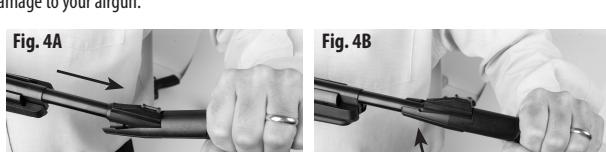
**CAUTION:** Make sure you do not pull the trigger while cocking the airgun or with the barrel in the down position. This may cause serious damage to the air pistol.
