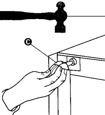
Insert casters **C** into holes at corners of dishwasher. Lightly tap casters with a small hammer until they lock in place.
