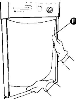
Bow door panel and insert other side door panel into door frame **F**.
