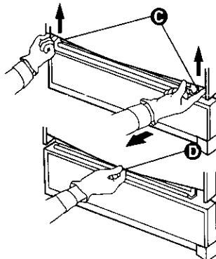
Lift door panel at outer edges **C**. Use one hand to bow bottom of panel **D**. Remove panel. Do Not remove spacer.
