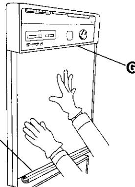
Push in on door panel near the top and slide panel and spacer up inside bottom of control console **G**, allowing panel to rest on channel **H** at bottom of door.
