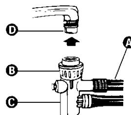
Turn on the hot water faucet until water is hot. Turn faucet off. Pull inlet/drain hose **A** from the storage compartment. Pull down on locking collar **B** and push hose connector **C** over end of faucet adapter **D**. It will snap into place. Release locking collar.
