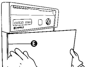
Insert one side of door panel, with desired color facing out, into one side of door frame **E**.
