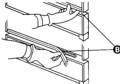
Insert finger under one end of retainer **B** and pull retainer towards you in a peeling action. Set retainer aside.
