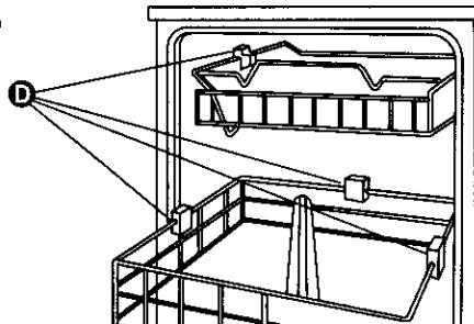
Stand dishwasher upright. Open door and remove beaded foam shipping pieces **D** from racks. Close dishwasher door. Latch dishwasher door shut.
