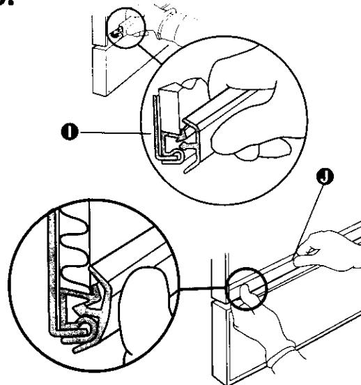
Snap one end of retainer into channel as shown **I**. Push inward while sliding thumb along full length of retainer **J**.
