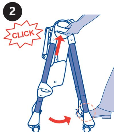
2. Stand at the back of the highchair and hold the two side joints, then press the open/close buttons. At the same time, open the Highchair legs using your foot, until an audible click is heard, signalling that the legs are locked in the open position (diagram 2).
