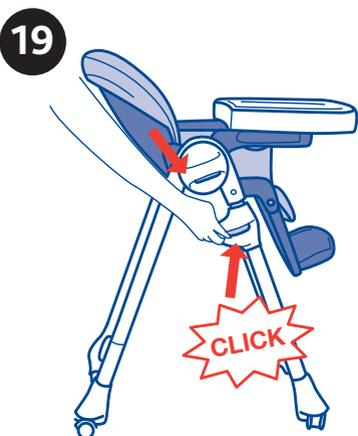
19. To lower the seat: Press the two side buttons simultaneously and lower the seat, until the desired height is reached (diagram 19).
