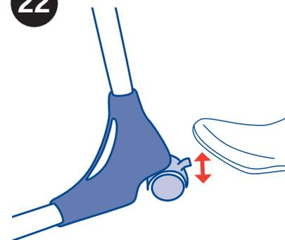
22. To apply the brakes, lower the wheels locking levers. To release the brakes raise the wheels locking levers (diagram 22).
