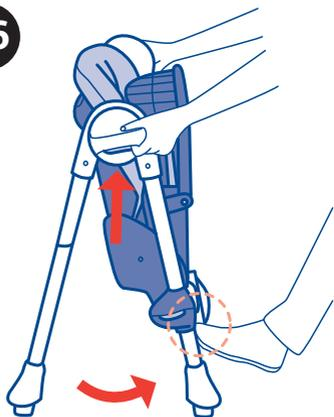
26. Press the buttons at the center of the side joints and, at the same time, close the legs of the Highchair using your foot (diagram 26A).
