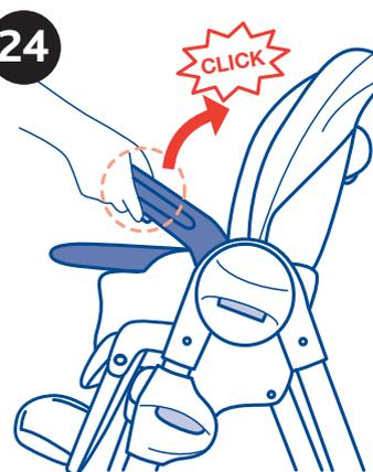
24. Raise the armrest in a vertical direction by pressing the buttons located on the lower part of the arm rests, until an audible click is heard (diagram 24).
