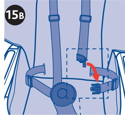
15B. Attach the shoulder harness to the waist belt clip. Hold the waist belt clip stationary and line up the arrows on the shoulder harness clip and waist belt clip. Push the shoulder harness clip down into the waist belt clip (twisting motion), it will click into place.
