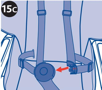
15c. Insert the waist belt clip into the crotch strap buckle, it will click into place. The harness straps can be adjusted to better fit your child (diagram 15D).
