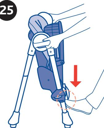
25. Lower the seat by pressing the two side buttons at the same time, as shown in the diagram 25.
