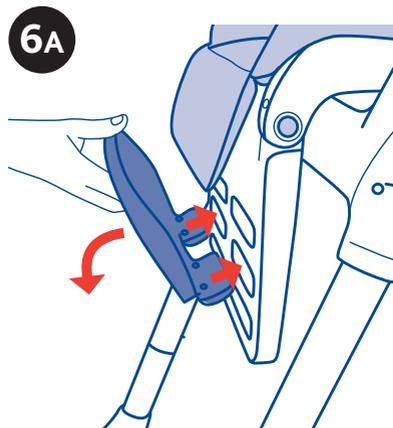
6. Insert the footrest, turn it until the use position is reached, and lock it into position (diagram 6A). The footrest can be adjusted to 3 positions. Remove the footrest and fit it at the desired height (diagram 6B & 6C). Turn the footrest until the new desired use position is obtained, and lock it into position.
