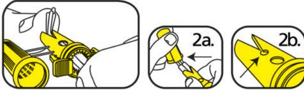
Insert wires through flexible sealing fingers and bend bare wire ends together into one "V-Channel." When connecting heavy solid wires, use bending sleeve / depth gauge on outer sleeve of connector (see illustration 2a). For larger connections (e.g. three #12 wires, or equivalent, or more), bend wires into the V-Channel with round hole at bottom (see illustration 2b); pull folded group of wires downward into this hole at bottom of "V."
