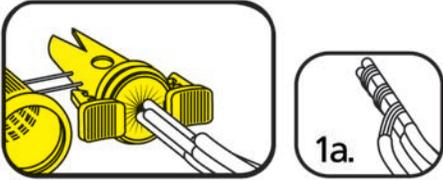
Strip wires 1" and group bare wire ends together. Do not pre-twist solid wire. You must pre-twist stranded wire. If using both wire types, you must wrap stranded wire around untwisted solid wires (see illustration 1a).
