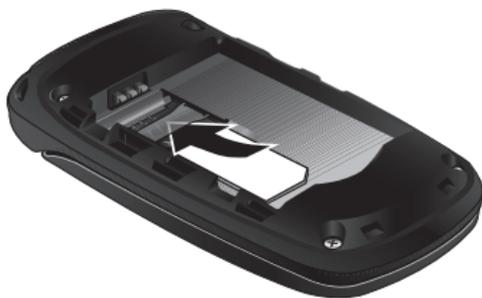
3. To remove the SIM, slide it gently out of the socket.
