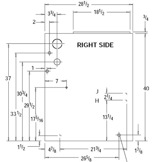
**NOTE:** Evaporator "A" coil drain pan dimensions may vary from furnace duct opening size. Always consult evaporator specifications for duct size requirements. Furnace is designed for bottom return or side return. Return air through back of furnace is NOT allowed.
