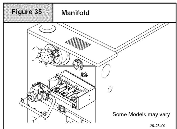
9. After reassembling, turn gas on and check all joints for gas leaks using a soapy solution. All leaks must be repaired immediately.
