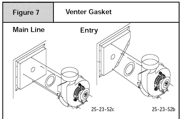
7. Tighten the three (3) or four (4) screws that secure the venter assembly to the collector box. Do not tighten screws enough to compress venter gasket.
