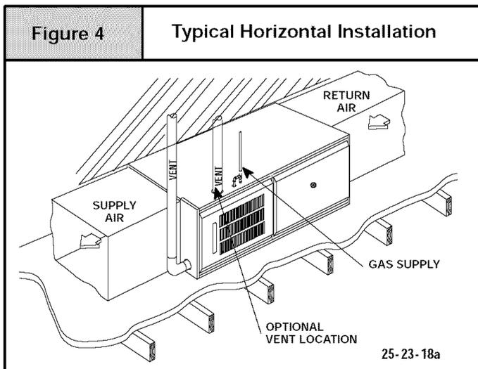
If the furnace is to be suspended from the floor joists in a basement or crawl space or the rafters in an attic, it is necessary to use steel pipe straps or an angle iron frame to attach the furnace. These straps should be attached to the furnace bottom side with sheet metal screws and to the rafters or joists with bolts. The preferred method is to use an angle iron frame bolted to the rafters or joists.
