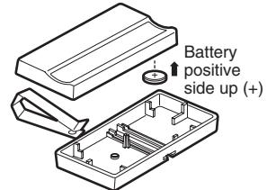
The lithium batteries should produce power for up to 5 years. To replace, pry open case with visor clip or screwdriver, as shown. Insert batteries *positive side up* (+).
