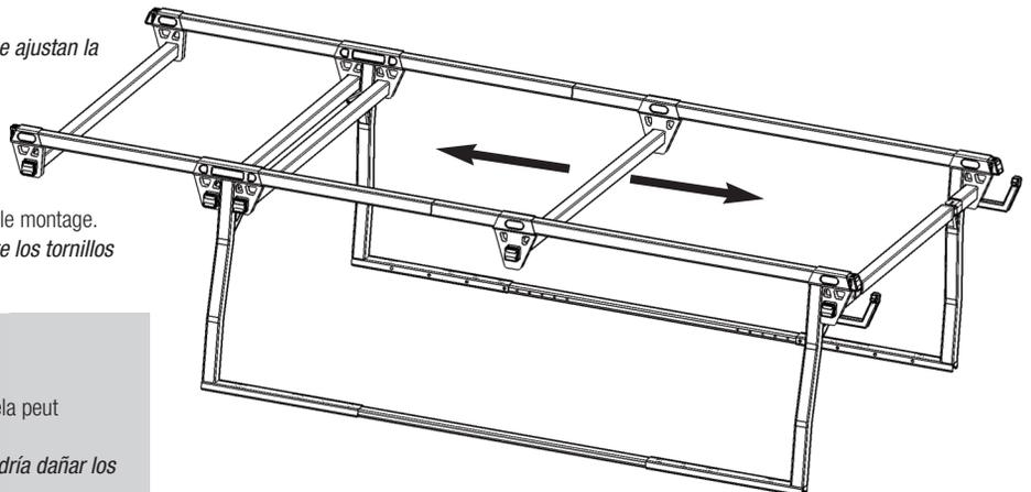
**NOTE: Do not over tighten locating screws as this may damage the upper side tubes.**
