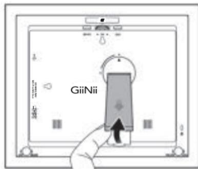
2. To place the Picture Frame horizontally or vertically, you can rotate the back stand by aligning the triangle mark with the rounded points (1 or 2).
