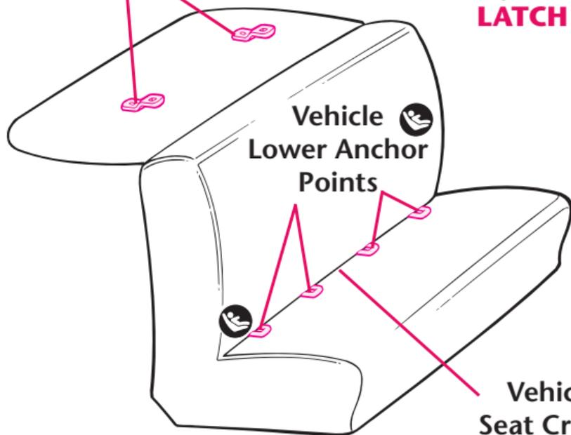
Typical seat in a passenger vehicle. Other vehicle types may have different **LATCH** locations.
