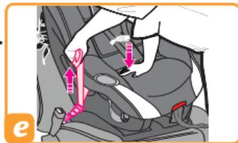
7. Hold seat and pull front to back and left to right at belt path to check for secure installation **(f)**. The child restraint should not move side to side or forward more than 1 inch (2.5 cm).
