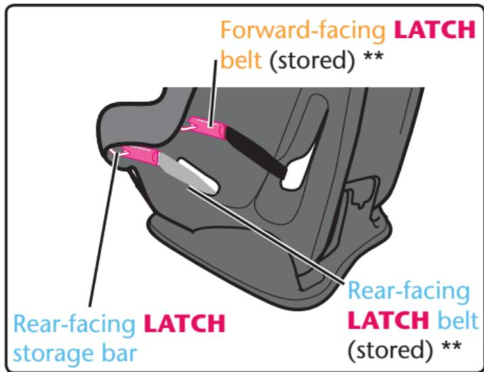
\*\*United States Federal Motor Vehicle Safety Standards have defined a system for installing child restraints in vehicles. The system is called **LATCH**. **LATCH** may **ONLY** be used **IN PLACE** of vehicle belt if vehicle is equipped with **LATCH** anchor points. Please refer to vehicle owner's manual for **LATCH** locations in vehicles.
