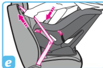
4. Hold seat and pull front to back and left to right at the belt path to check for secure installation. **(f)** The child restraint should not move side to side or forward more than 1 inch (2.5 cm). Vehicle lap belt **MUST** stay tight. If not secure, see “Vehicle Seat Belts” page 41.
