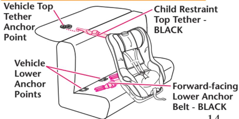
**LATCH** lower vehicle anchor points are defined as 11 inches (28 cm) from the center of one **LATCH** anchor to the center of another **LATCH** anchor.
