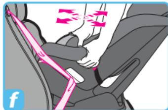
5. Check level indicator on child restraint. **Vehicle must be on level ground** and child in child restraint when checking level indicator.
