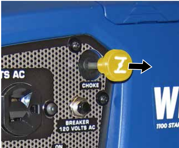
Figure 29 – Choke Knob (WH1000i Shown)
