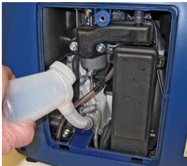
Figure 37 – Adding Engine Oil
