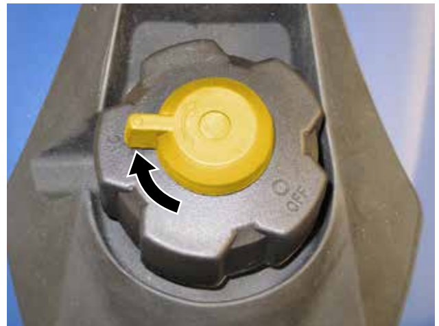
Figure 27 – Fuel Tank Vent
