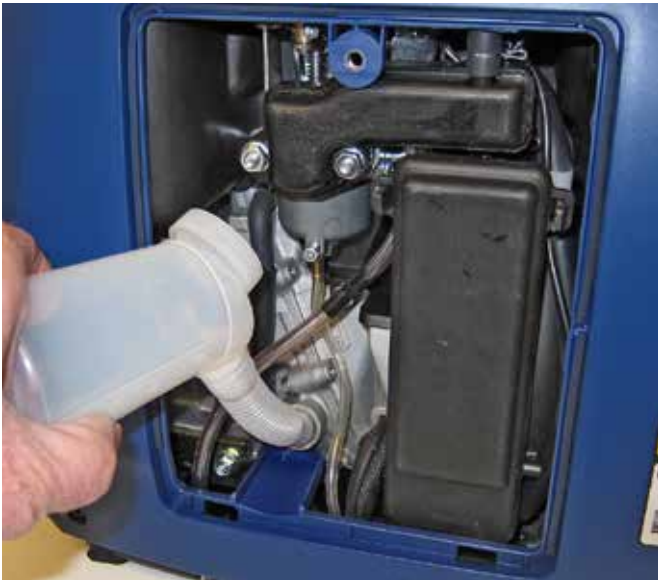
Figure 19 – Adding Engine Oil
