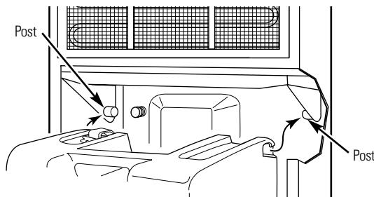
Make sure the bucket is locked securely in place by pressing down on the upper back edge of the bucket. It will be firmly seated when properly installed.
