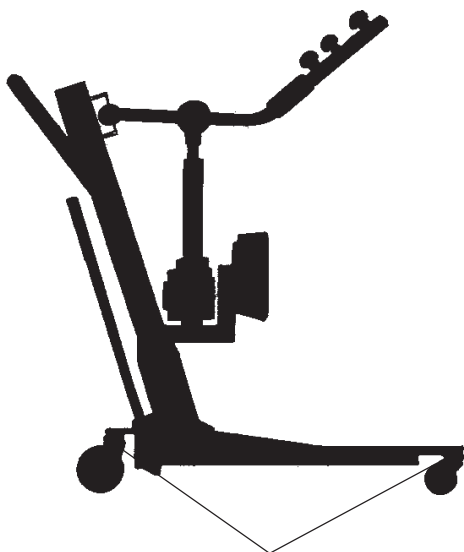
Lubricate the Bearings in the Caster Swivels
