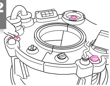
Unscrew three leg bolts and remove tray from legs.
