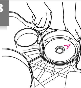
Put tray together as shown. Make sure "A" is over "B" and screw together.
