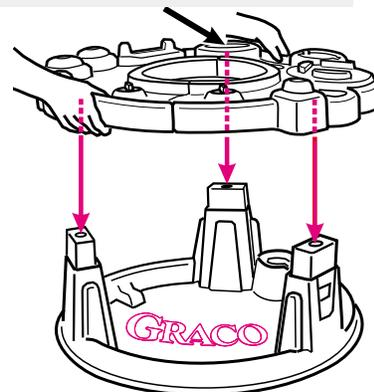
Check that bolts are secure by pulling up on tray.
