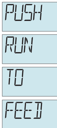
Figura 3-7 Alarma PUSH RUN TO FEED
