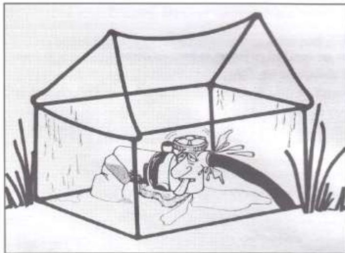
Lack of adequate ventilation causes overheating.
