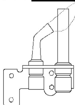
Pilot is located on side of burner
