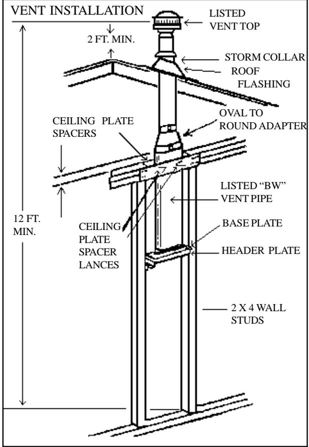
FIGURE 2 - VENT INSTALLATION
