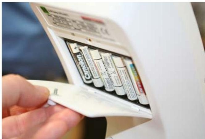
Figura 3-9. Batteries in Battery Chamber
