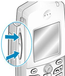
In idle mode, you can adjust the key tone volume using the same keys.
