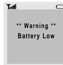
When the battery becomes too weak for the phone to operate, the phone switches off automatically.
