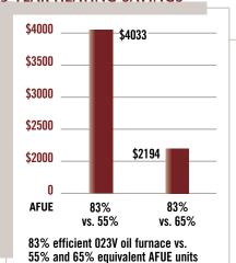
This chart depicts potential energy savings you can expect from the 023V furnace versus older furnaces with lower efficiency ratings. Criteria used in this example are 2,000 full-load heating hours, with a 80,000-Btuh heating design load and \$1.90 per gallon for oil. Your actual savings will vary depending on the weather, local fuel rates and your lifestyle.
