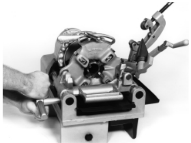
Figure 7 – Threading Pipe with No. 811-A Die Head
