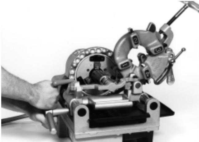
Figure 6 – Reaming Pipe with No. 323 Reamer
