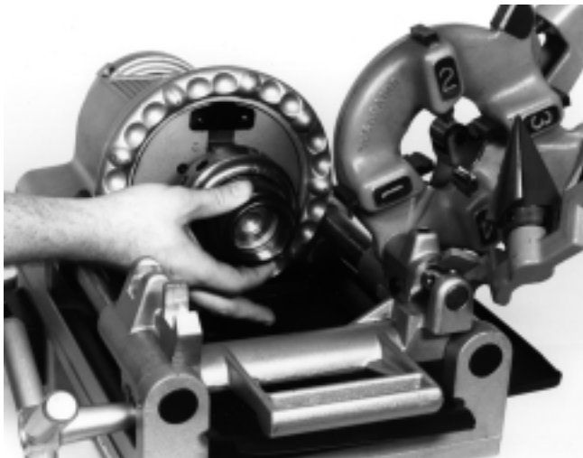
Figure 14 – Installing Nipple Chuck Adapter
