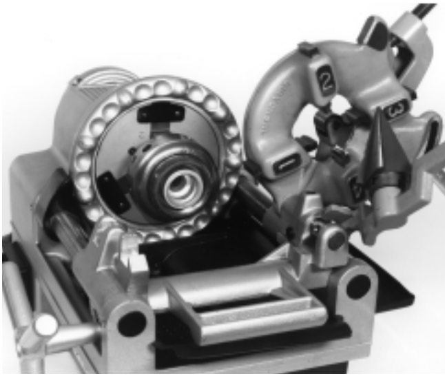
Figure 12 – Place Nipple Chuck Body in Power Drive
