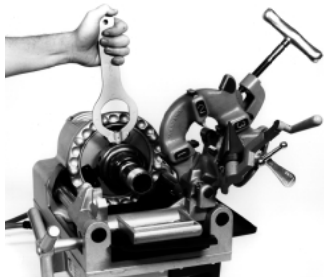
Figure 16 – Releasing Threaded Nipple from Adapter
