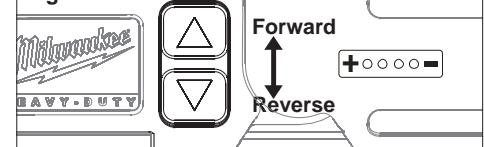
Press and hold the forward/reverse switch up for forward rotation, and down for reverse rotation. The switch will automatically return to the center, OFF position when it is released.
