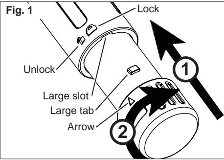
Line up the large and small tabs on the battery with the large and small slots in the tool opening. Slide the battery all the way into the tool. Turn the battery clockwise to lock it in place. The arrow on the battery will line up with the on the tool.
