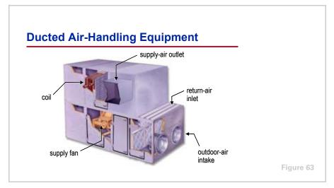
One of the best examples to demonstrate the complexity of gathering complete and accurate sound data is air-handling equipment. This involves any type of HVAC equipment that contains a fan and is used to condition and move air through a duct system.
