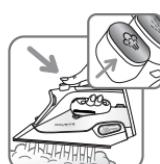
Press the burst of steam button to generate a powerful jet of steam. Wait a few seconds between each shot before pressing the button again.
