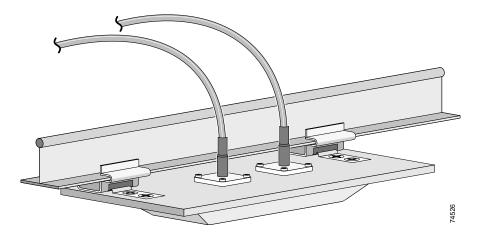
Step 7 Route the antenna cables into the space above the ceiling grid and connect them to the device or extender cables.
