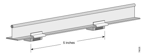
Step 6 Grasp the antenna with one hand and the track with the other while inserting the antenna's mounting clips into the ceiling mounting clip adapter until they can go no further as shown in the following illustration.
