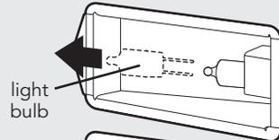
3. Replace with halogen bulb using volt and wattage requirements listed on glass cover.
