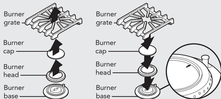
**Note:** When replacing burner head, arrow must be pointing towards back of range.
