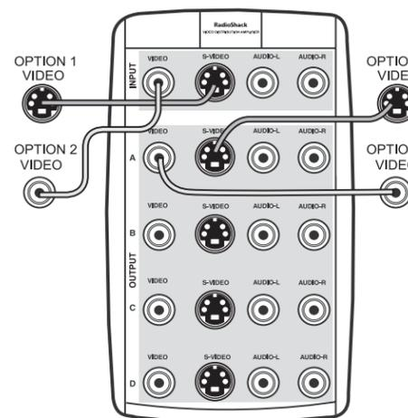
1. Connect the input device video cable.
