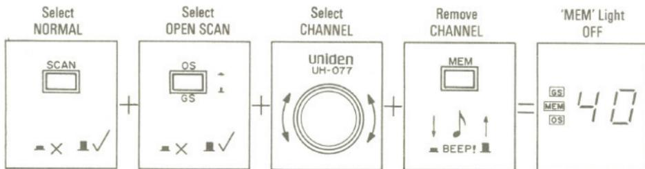
The selected channel has now been removed from the scan group and will not be included when scanning has commenced and the **MEM** indicator will not light on that channel.
