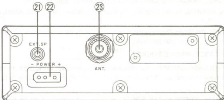
21. **EXTERNAL SPEAKER:** The External Speaker Jack is used for remote receiver monitoring. The external speaker should have 8-ohm impedance and be rated to handle at least 4.0 watts. When the external speaker is plugged in, the internal speaker is automatically disconnected.
