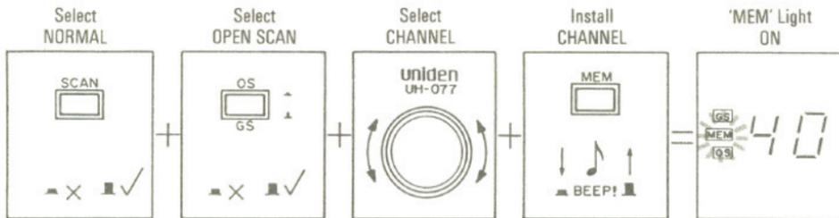
When you have finished, rotate the channel switch and notice that the **MEM** light is indicating which channels are programmed and which have been removed.
